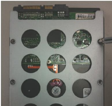
4. Push the tray back in the unit and press down the black bar to secure the tray
