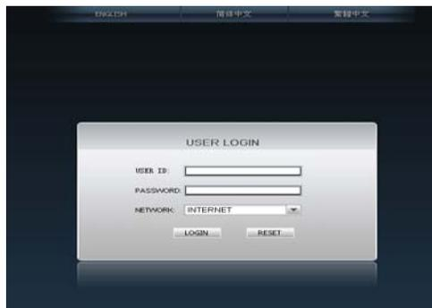
Select English interface from the top left side. Input correct password if password is enabled to enter the system. The password is the same as the one set in DVR.
