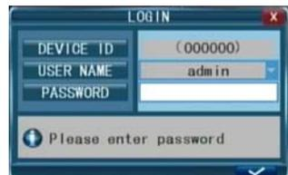
You can login from the LOGIN window as shown as previous fig. Select user name and user password via numeric key-board. You can access the main menu by pressing [] if the password is enabled.
