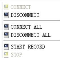
You can open, shut down and start this channel's record using the shortcut menu.
