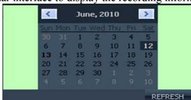
The highlighted date indicates that video was recorded on that day. Click on a date to search the recording file list of that day. For example, the above fig shows that June, 12<sup>th</sup>, 13<sup>th</sup> have recorded video when it shows on bold, and current search date is June 12<sup>th</sup>. Select channel and type at the bottom of the calendar. Click “SEARCH” and the result will display as follows.
