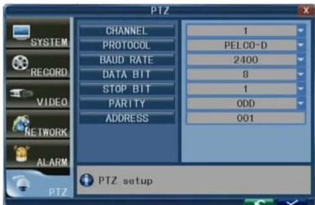
Move the cursor to [PTZ] (the icon will be highlighted when selected) and press [Enter] to access setting interface. You can setup the parameters for each channel separately.
