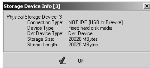
Fig.4. DVR Storage Device Information Window
